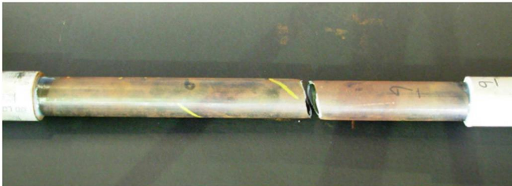
Figure 10. Failure location for specimen 9.
