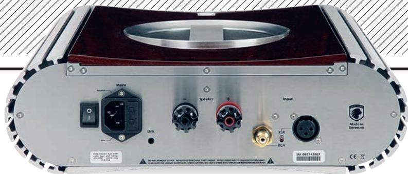
ABOVE: Simplicity itself – single-ended (RCA) and balanced (XLR) inputs are selected by a small toggle switch while WBT NextGen 4mm terminals serve speaker outputs
