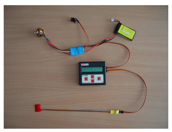
Color dot on the controller marks signal pin, which must be always connected to orange wire of the extension cable like we explained earlier.
