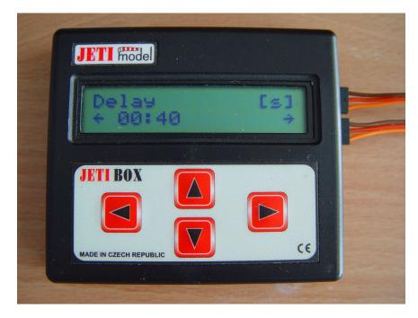
It is "delay". Buttons right and left can change its value. Next parameters are accessible again by "down" button.
