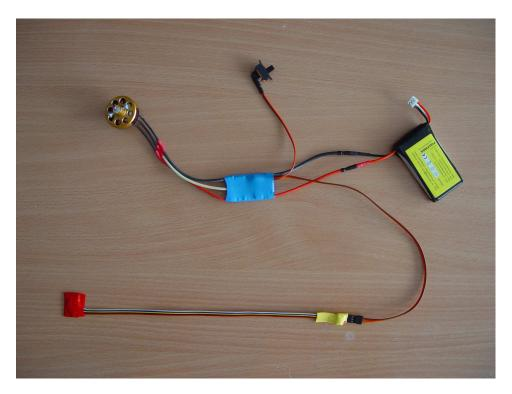
Simply connect the controller to ESC so that the point on controller connector goes to orange signal wire of ESC:
