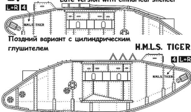
2. Late version with cylindrical silencer
