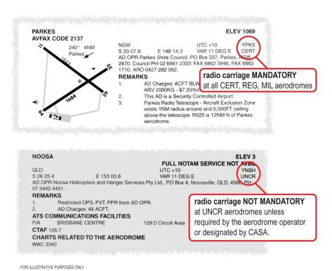
Figure 1 – Radio carriage requirements as depicted in ERSA
