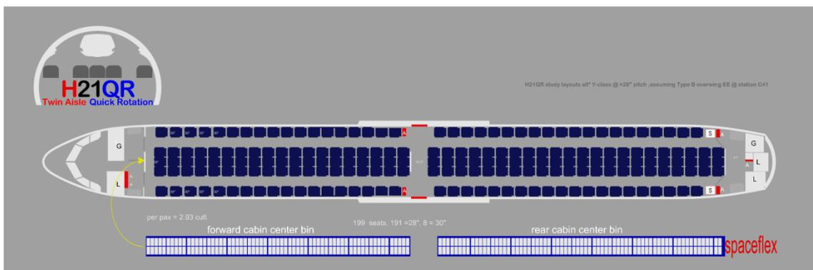
Here the aisle pax density is 1.48 sqft/pax, or 240 % better vs A321. Needless to say, whether with the current A32X Series' "Enhanced" interior (cabin carry-on OHSV - overhead stowage volume = 405 cuft total in A321 or only 1.7 cuft/pax in Hrnkova's outraged 236-pax configuration) or with the ISIS (Zodiac Aerospace) cabin interior option, @ peak-hour (≈ 100 %) cabin load-factors, eight out of the
