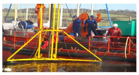
Std Height Ranges Barrel length - 3-6m (frame length of 4.2m-7.2m)
