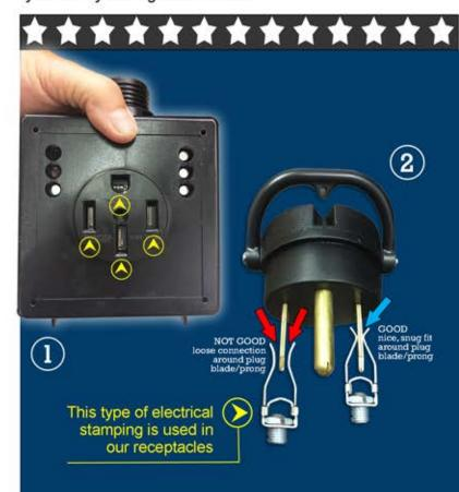
A Good Fit... Another problem we often see is a loose, sloppy fit. It is imperative the plug maintain a snug fit when plugged in. You may be tempted to wiggle the plug loose when disconnecting but over time this will compromise the connection making your unit susceptible to heat damage.
