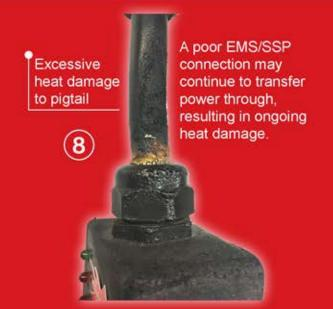
Inspecting your electrical connections on a daily basis could help prevent damage to your unit.
