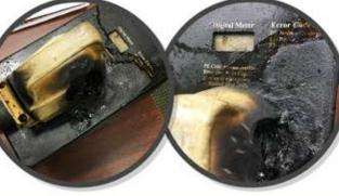
A poor connection forces the voltage to arch creating extreme heat which results in external melting.
