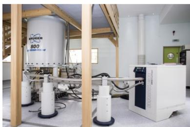
800 MHz NMR spectrometer, SoC.
