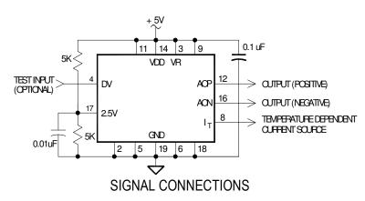
The 2.5V input (pin 17) may be driven from a resistive divider.
