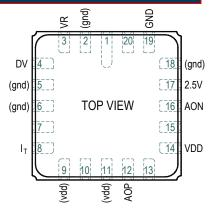
**DV (input):** Pin 4. Deflection Voltage. Normally left open. A test input that applies an electrostatic force to the sense element, simulating a positive acceleration. The nominal voltage at this pin is ½ VDD. DV voltages higher than required to bring the output to positive full scale may cause device damage.
