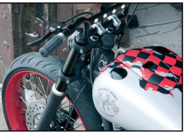
five light 'lenses' in a brushed aluminium finish that ties in with the handlebar inserts. Don't go looking for the wires: they pass through to the headstock through the headlamp bracket and bottom yoke. All other lighting is taken care of by Kellermann's mini LEDs – barely visible at the front, and completely invisible at the back in the main shots because they were fitted a couple of days after the shoot: check out the detail shots for them, and the billet bar that keeps them neat.
