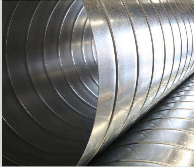
Common methods of sealing spiral ductwork include: standard slip-fit connections which require the application of joint sealant, flanged connections with an applied gasket, or factory-applied gaskets which effectively seal spiral duct connections without the use of sealants.
