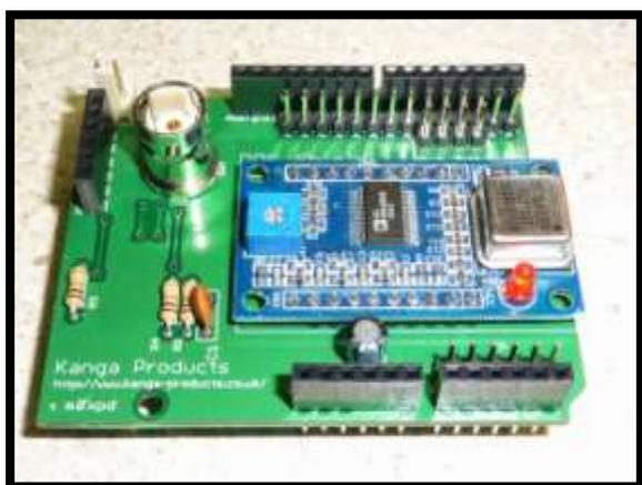
The m0xpd Arduino DDS shield provides a convenient interface between an AD9850 DDS module and an Arduino, opening up the benefits of this flexible “*Electronics prototyping platform*”. The shield makes the DDS Module easy to configure (through software) and to control (through familiar, everyday interfaces such as Keypads, Displays and Rotary Encoders).
