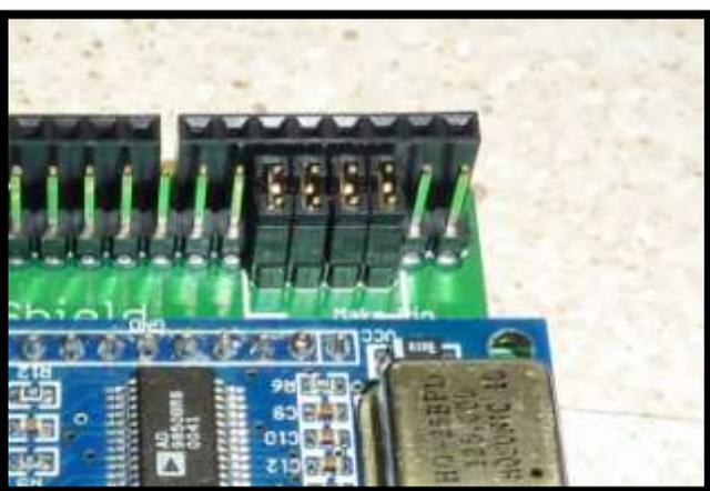
Conventional male header plugs are used to make easy connections between the Arduino’s input/output pins and the DDS module. These headers, along with the stackable headers, are seen fitted in the photo right.
