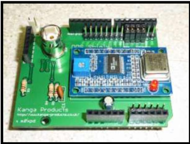
Gently offer the DDS Module to the DDS Shield PCB in the orientation shown here in the picture. It may be necessary just to slightly adjust the odd pin to ensure correct alignment.
