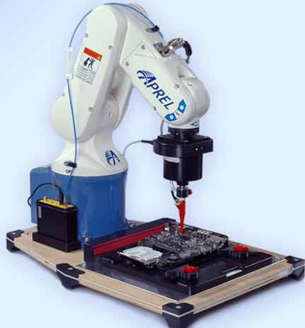
EM-ISight with the far-field approximation module is a complete solution for the assessment of electronics during design, development, optimisation, analysis, quality control & management.
