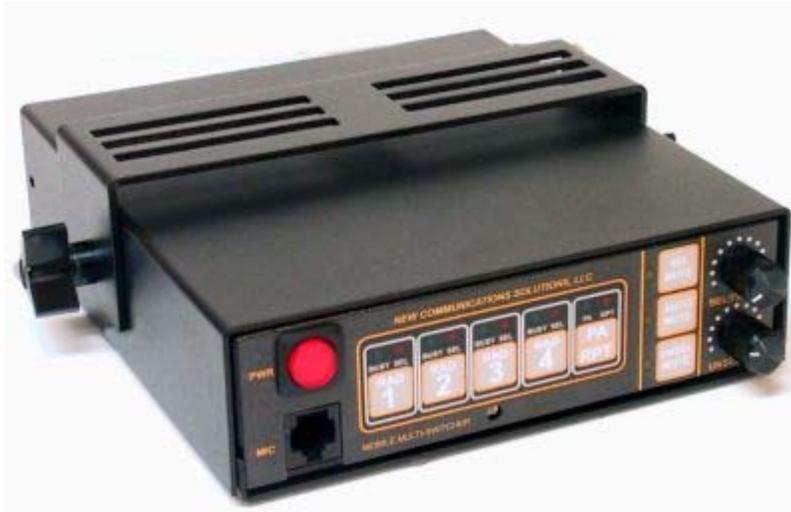
The NCS-C250 Mobile Multi-Switcher is an interoperability solution suited for First Responders that utilize multiple radios such as police, fire and EMS personnel. However, many customers have purchased the unit for dispatch purposes. The unit connects four radios to one microphone and two speakers. Specific features such as crossband repeating of up to 4 radios (VOX operated), Select/Unselect audio control and muting, and PA output make the unit more than a "microphone switch".
