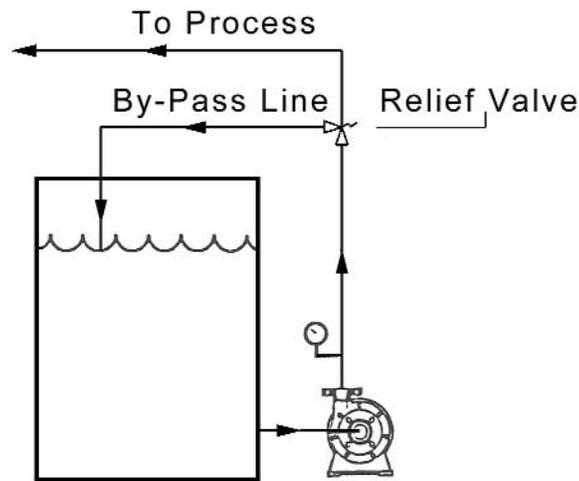
**Figure 2:** By-pass Configuration
