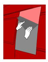
4. When edges and corners are resqueegeed, make sure the material is fixed on the edges of the corrugation (see below), and work your way around the entire corrugation, just fixing the edges.
