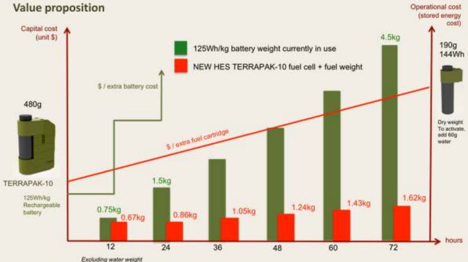
Lithium Battery vs SOLDIERPAK weight comparison assuming 10W continuous power
