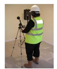
Fig. 1 Sound test being carried out
