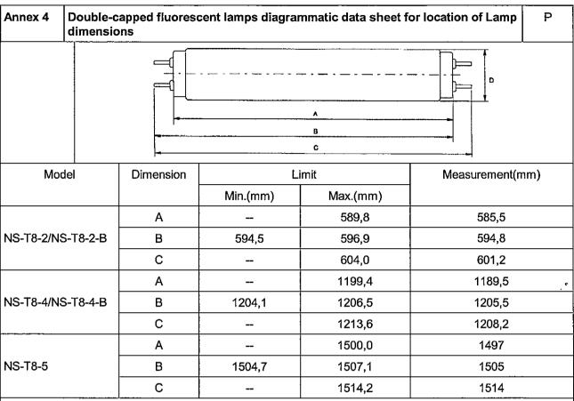
For NS-T8-2 /NS-T8-2-B, the limits are referred to the dimensions of fluorescent tube of T8 18W or 20W. For NS-T8-4-B /NS-T8-4-B, the limits are referred to the dimensions of fluorescent tube of T8 36W, 40W. For NS-T8-5, the limits are referred to the dimensions of fluorescent tube of T8 58W or 65W.
