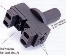
Unit is very easy to use — simply set gap between jaws 1/8" smaller than stock size. As the bar puller slides over the bar along the x-axis, the jaws compress heavy-duty internal die springs to provide high gripping force. The turret then retracts along the z-axis, pulling the bar out the desired position.
