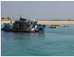
A Model 5012 LP removes silt from channels at a
