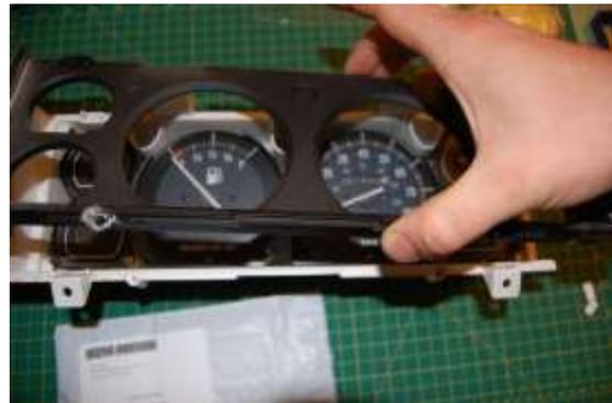
5. Choose your first gauge. You may find that the gauges are dusty... clean with a dry soft cloth and an air-duster. Remove the 2 screws (some may also have washers) and set these aside. We recommend one of the smaller gauges first, as the larger ones have an extra step and obstructions.
