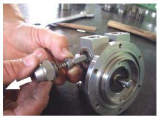
14) Remove the screw from the external magnet.
