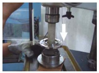
12) Pay close attention to small pins inside the holes on the shaft when disassembling the cartridge.
