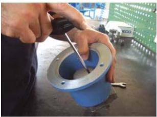
5) Pull the internal assembly from the pump casing.
