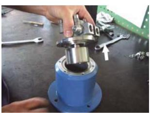
6) Remove the dowel pin connecting the internal magnet to the pump shaft.
