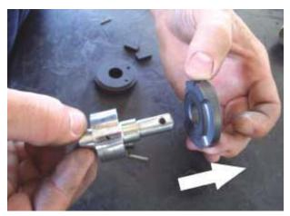
13) Remove hex nut from the pump casing and pull out the by-pass components.
