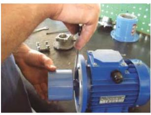
15) Using an extractor pull out the external magnet from the motor shaft.
