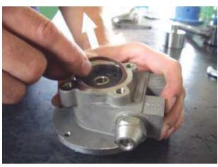
10) Before removing carbon cartridge and rotor from pump casing, it may be helpful to heat the assembly up to a temperature of 300-350°F.
