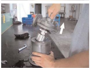
6) Remove hex bolt connecting internal magnet to the pump shaft.
