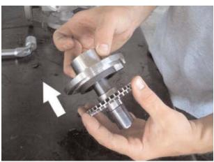
9) Remove the retaining ring from the shaft.
