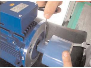
17) Using an extractor pull out the external magnet from the motor shaft.
