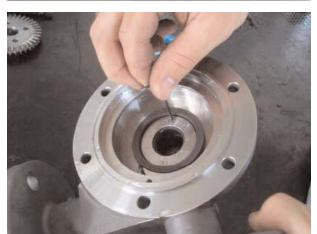
14) Remove the two screws from the volute ring and pull out the special carbon ring.
