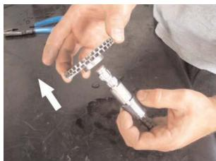
13) Remove the two screws from the pump casing and pull out the special carbon ring.
