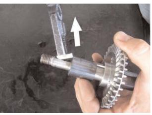
11) Pull out the two sleeve bushings from the shaft.
