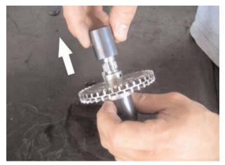
12) Pull out the impeller.
