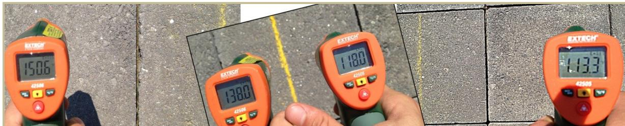
This photo compilation is an example of the cooling effect of ThermaPAVER® while heating water. The left side of the yellow line is a control zone without ThermaPAVER® (138°-150.6°). A ThermaPAVER® system is actively running on the right side of the yellow line (113°-118°). Far left and right readings are 16" apart, indicating a 36.76°f differential. The middle readings are only 3" apart on the same paver, at the same time, indicating a 20°f differential.
